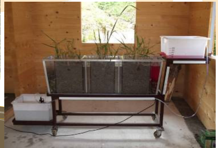
DEMONSTRATION MODEL OF CONSTRUCTED WETLAND
